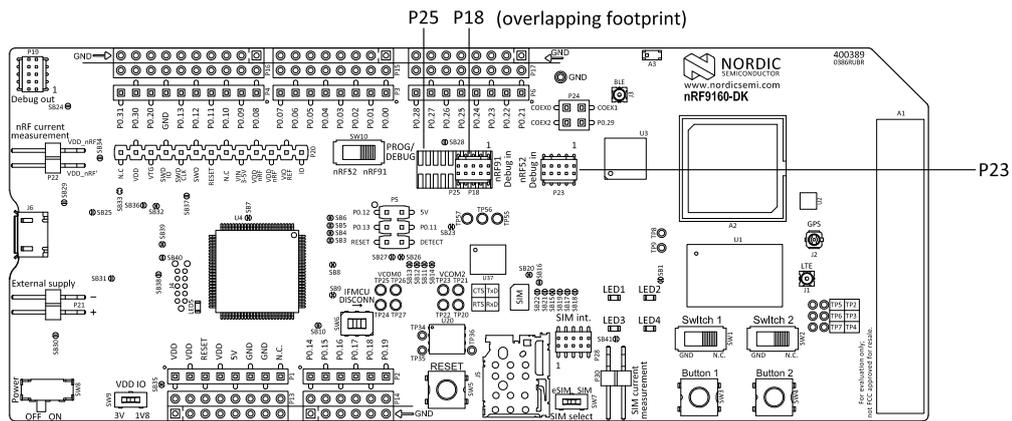
Figure 21: Debug input connector and trace footprint
