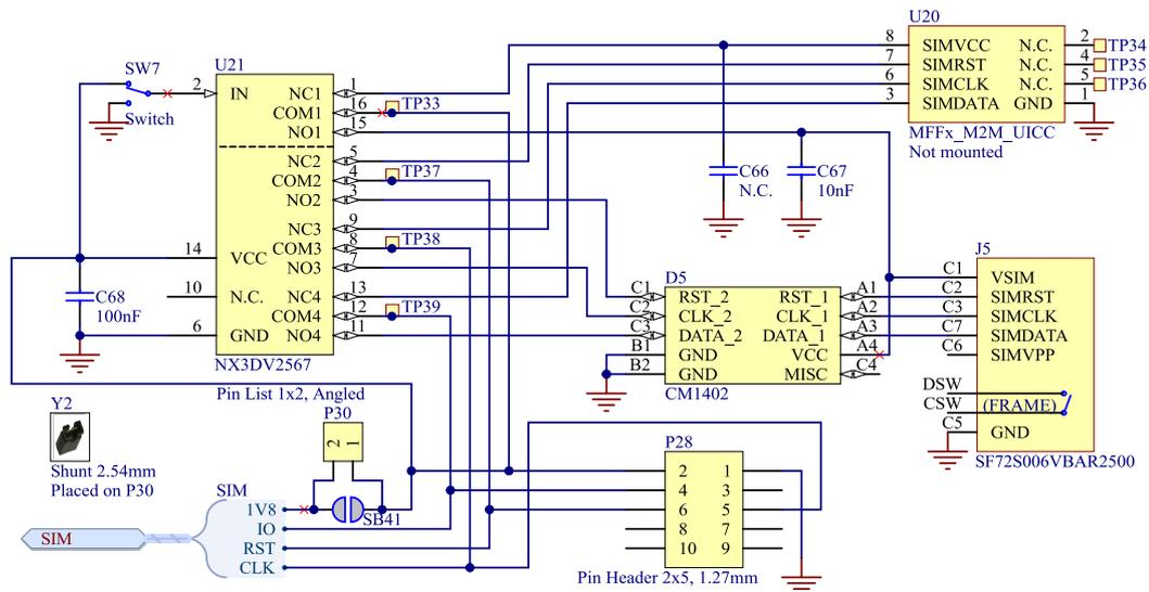
Figure 29: SIM card connector, eSIM, and selection switch
