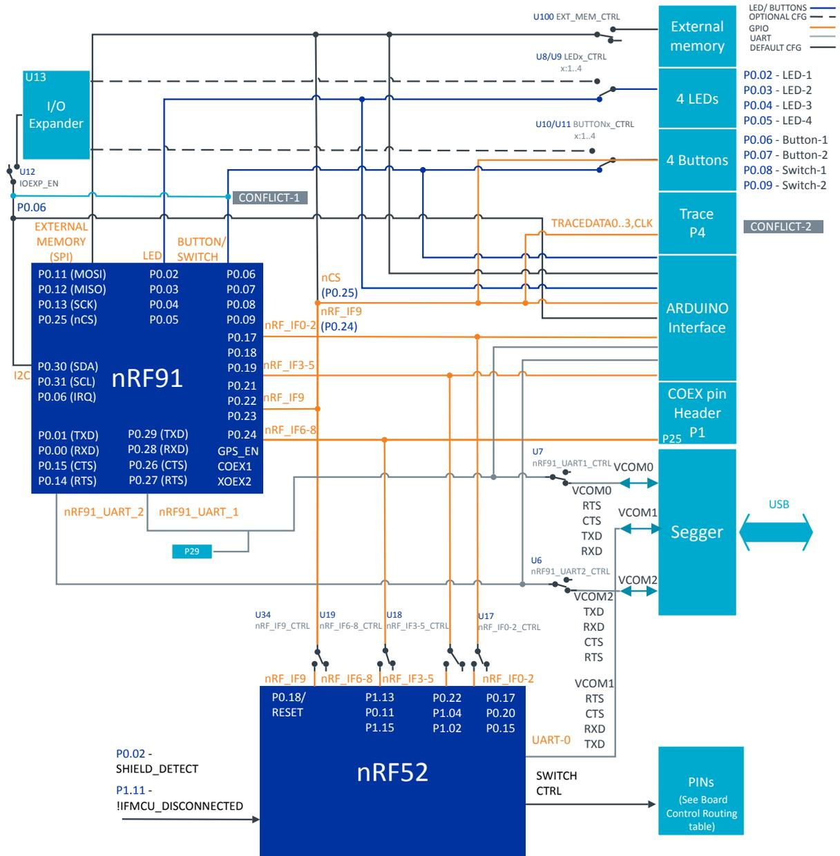
Figure 16: nRF9160 DK board control
