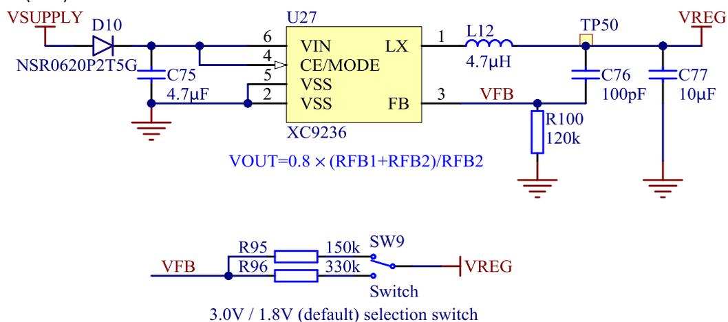
Figure 10: VDD buck regulator and selection switch
