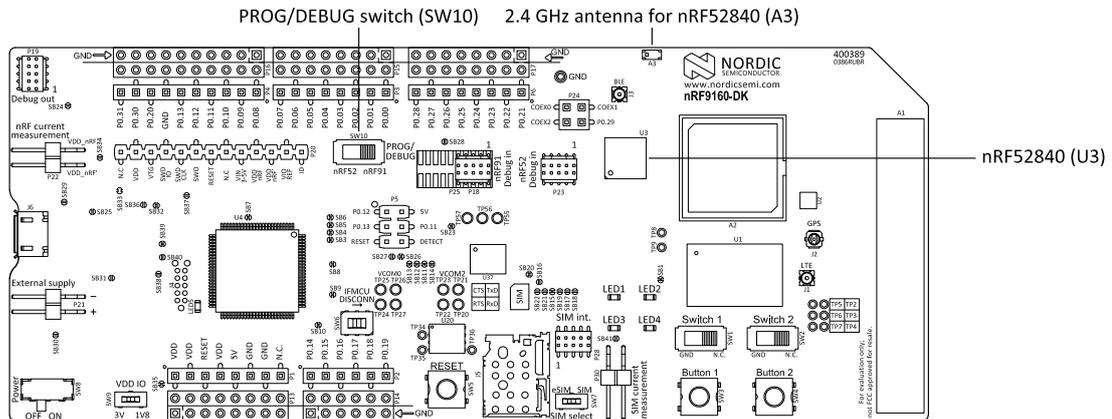
Figure 15: nRF52840 SoC on the nRF9160 DK
