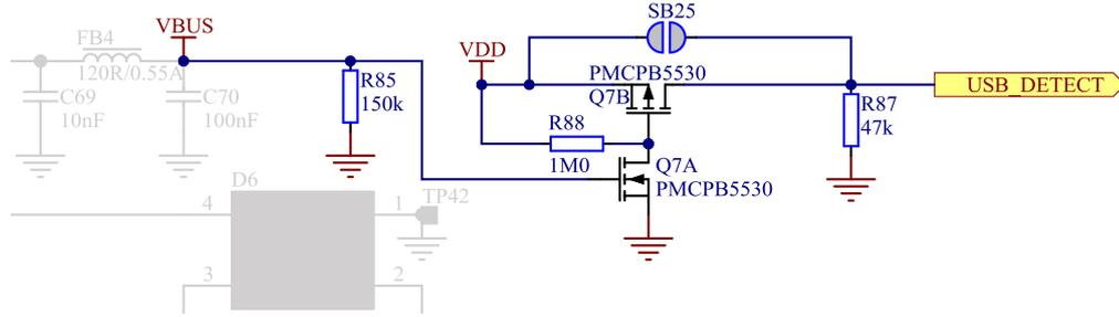
Figure 4: USB detect switch
