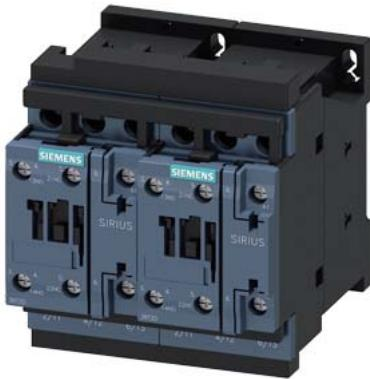
Reversing contactor assembly AC-3, 5.5 kW/400 V 110 V AC 50 Hz/120 V 60 Hz, 3-pole Size S0, screw terminal electrical and mechanical interlock
