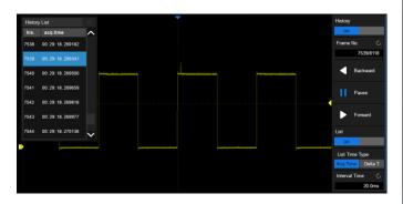
History function records up to 90,000 triggered waveforms (frames). This is done continuously in the background, so the history waveforms can be played back at any time to find and analyze past events. Serial decode, zoom and cursors measurements can be used.
