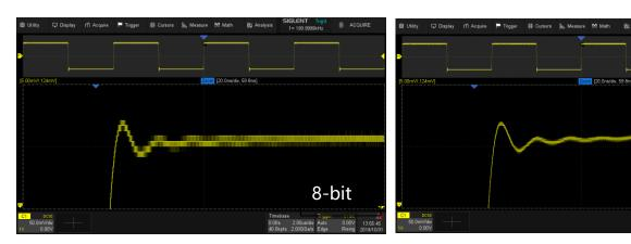
10-bit mode combined with Zoom shows you more details and less noise on the waveform.
