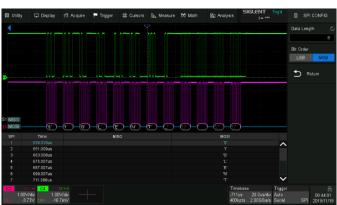
In addition to the decoder lanes correlated to the waveform, bus protocol information can be displayed in tabular form.  $I^2C$ , SPI, UART, CAN, LIN, CAN FD, FlexRay,  $I^2S$ , MIL-STD-1553B, SENT and Manchester are supported.
