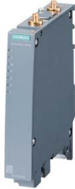
IWLan client, SCALANCE W734-1, RJ45, 1 radio, 2 R-SMA antenna port, iFeatures support via key plug, IEEE 802.11a/b/g/h/n, 2.4/5GHz, gross data rate 300 Mbit/s, 2x RJ45 max. 100 Mbit/s, PoE integrated 2-port switch, redundant 24 V DC, terminal block, IP30, -20... 60 °C, plug slot WPA2/802.11i/e, observe national approvals! CERT ID: MSN-W1-RJ-E2, scope of delivery: Manuals on CD-ROM, German/English, 1x terminal block; only for operation in USA
