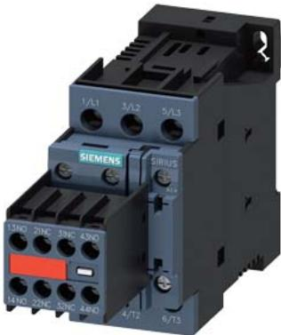
Power contactor, AC-3 38 A, 18.5 kW / 400 V 2 NO + 2 NC, 24 V DC with plugged-in diode combination, 3-pole Size S0, Screw terminal Captive auxiliary switch
