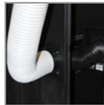
Exhaust duct accessory for Tripp Lite SRCOOL7KRM. Directs and disperses heat from the air conditioning unit through an upper vent into your facility's ventilation system.
