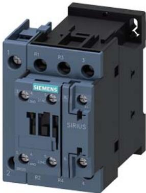
Contactor, 2NO + 2NC, AC-3, 11 kW, 110 V AC, 50 Hz, 120 V, 60Hz, 4-pole, 2NO + 2NC, Size S0, Screw terminal 1 NO + 1 NC integrated
