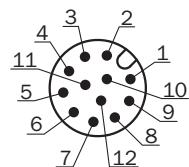
Connecting cable with male connector or M12 male connector, 12-pin, A-coded
