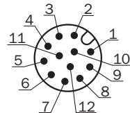
Cable with male connector M12, 12-pin, A-coded
