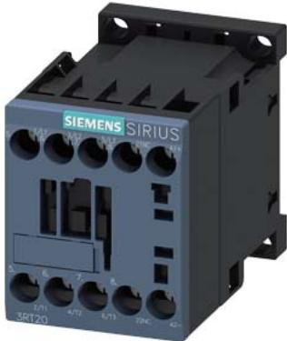
Power contactor, AC-3 7 A, 3 kW / 400 V 1 NC, 24 V DC 3-pole, Size S00
