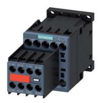
Contactor relay, 4 NO + 4 NC, 24 V DC, Size S00, screw terminal, Captive auxiliary switch, for SUVA applications
