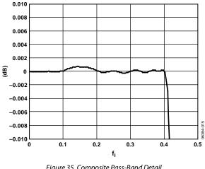
Figure 35. Composite Pass-Band Detail (Frequency Scaled to Input Sample Rate of Half-Band 1)
