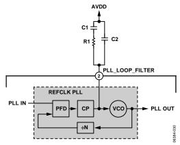
Figure 52. REFCLK PLL External Loop Filter
