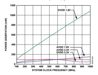
Figure 22. Power Dissipation vs. System Clock (PLL Disabled)
