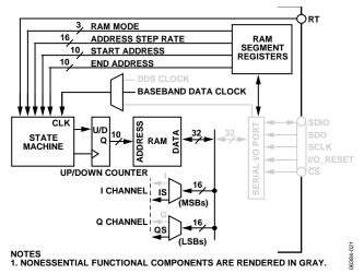
Figure 41. RAM Playback to Baseband Scaling Multipliers
