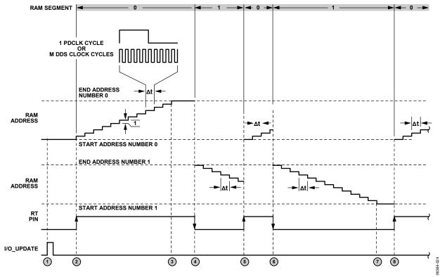
Figure 44. Bidirectional Ramp Timing Diagram
