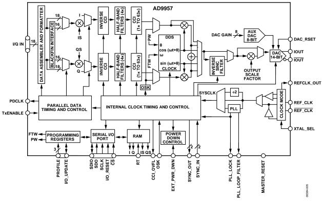
Figure 25. Detailed Block Diagram
