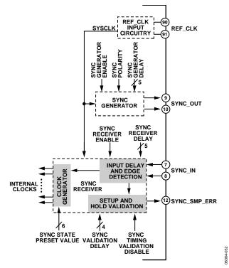
Figure 54. Synchronization Circuit Block Diagram
