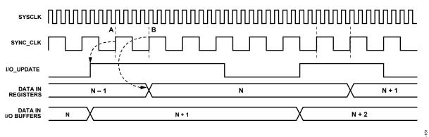
THE DEVICE REGISTERS AN I/O UPDATE AT POINT A. THE DATA IS TRANSFERRED FROM THE ASYNCHRONOUSLY LOADED I/O BUFFERS AT POINT B.
