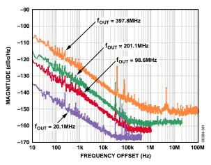
Figure 20. Residual Phase Noise, System Clock = 1 GHz
