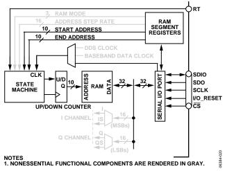
Figure 40. RAM Load/Retrieve Operation
