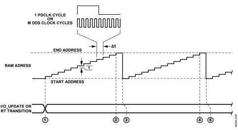
Figure 46. Continuous Recirculate Timing Diagram
