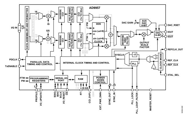
Figure 26. Quadrature Modulation Mode
