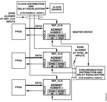
Figure 59. Multichip Synchronization Example
