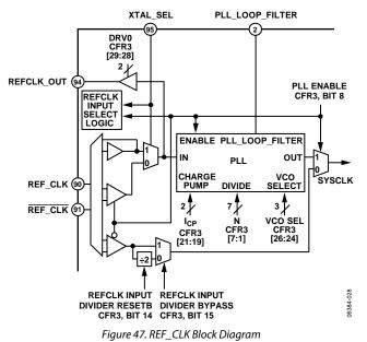
The PLL enable bit is used to choose between the PLL path or the direct input path. When the direct input path is selected, the REF\_CLK/REF\_CLK pins must be driven by an external signal source. Input frequencies up to 2 GHz are supported. For input frequencies greater than 1 GHz, the input divider must be enabled for proper operation of the device.
