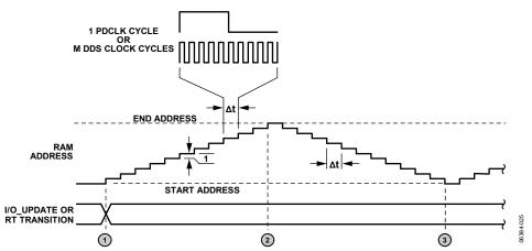
Figure 45. Continuous Bidirectional Ramp Timing Diagram
