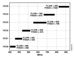
Figure 50. VCO Ranges Including Atypical Wafer Process Skew
