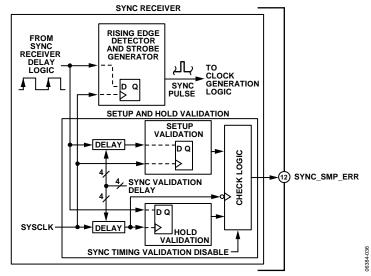
Figure 58. Sync Timing Validation Block
