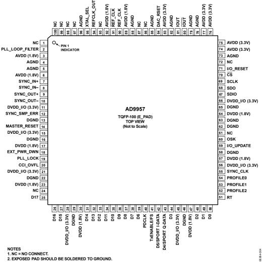
Figure 4. Pin Configuration
