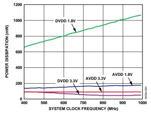
Figure 23. Power Dissipation vs. System Clock (PLL Enabled)
