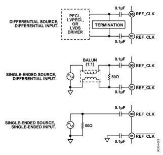
Figure 49. Direct Connection Diagram
