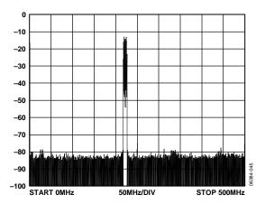
Figure 12. QPSK, 7.8125 Msymbols/s, 4x Oversampled Raised Cosine, a = 0.25, CCI = 8, Carrier = 222 MHz,  $f_5 = 1$  GHz
