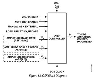
Four control register bits, the external OSK pin, and the entire 32 bits of the ASF register govern the operation of the OSK function. The primary control for the OSK block is the OSK enable bit. When this bit is set, the OSK function is enabled; otherwise, the OSK function is disabled. When disabled, the other OSK input controls are ignored and the internal clocks are shut down to conserve power.
