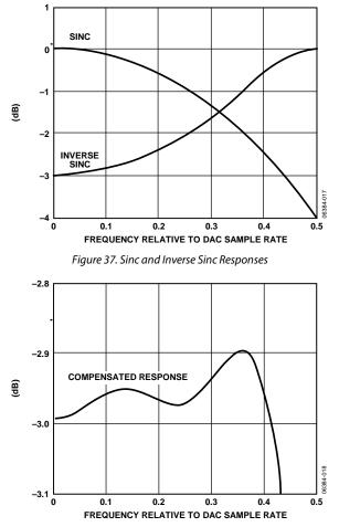
Figure 38. DAC Response with Inverse Sinc Compensation
