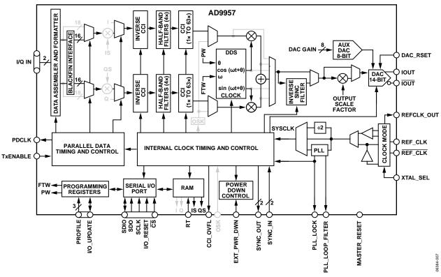
Figure 27. Quadrature Modulation Mode, Blackfin Interface
