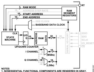
Figure 42. RAM Playback to Baseband Data Path
