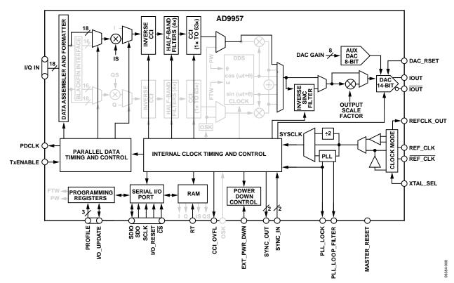
Figure 28. Interpolating DAC Mode
