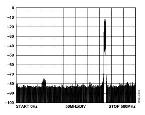
Figure 13. QPSK, 7.8125 Msymbols/s, 4x Oversampled Raised Cosine, a = 0.25, CCI = 8, Carrier = 372 MHz, fs = 1 GHz
