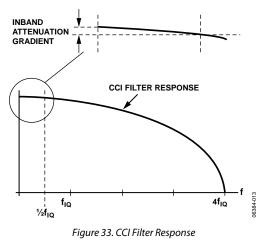
The product of the two responses yields an extremely flat pass band ( $\pm 0.05$  dB over the baseband Nyquist bandwidth) eliminating the in-band attenuation gradient introduced by the CCI filter. The cost is a slight attenuation of the input signal (approximately 0.5 dB for a CCI interpolation rate of 2, and 0.8 dB for higher interpolation rates).
