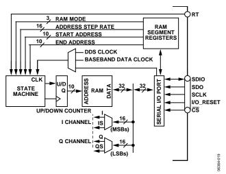
Figure 39. RAM Block Diagram
