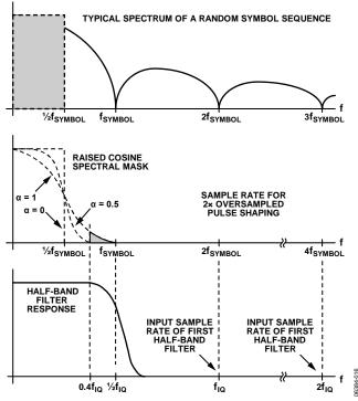
Figure 36. Effect of the Excess Bandwidth Factor (a)
