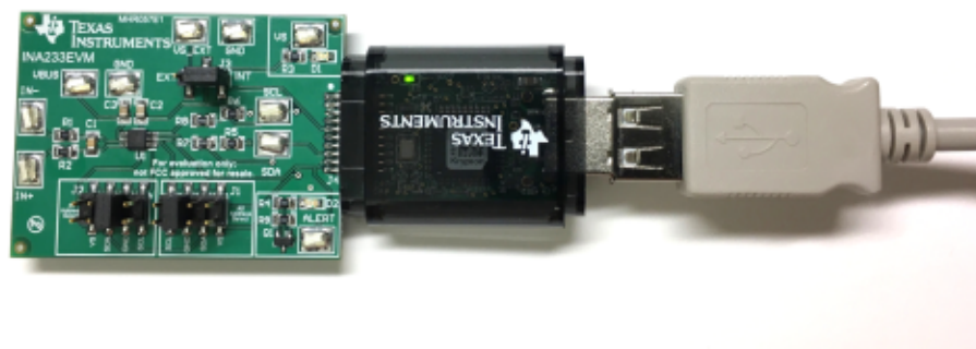
Figure 9. Connecting the INA233 Test Board and SM-USB-DIG Platform board
