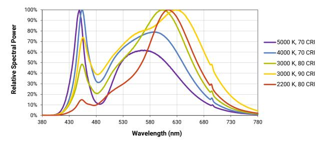
The following graph is the result of a series of pulsed measurements at 450 mA and T\_J = 85 °C.
