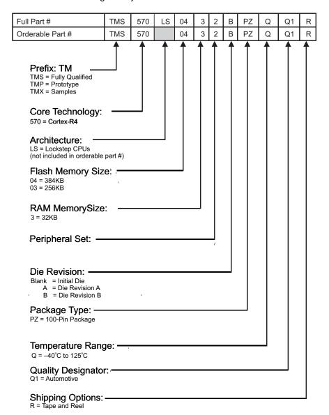
Figure 8-1. Device Numbering Conventions
