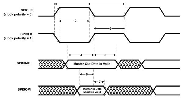
Figure 7-6. SPI Master Mode External Timing (CLOCK PHASE = 0)
