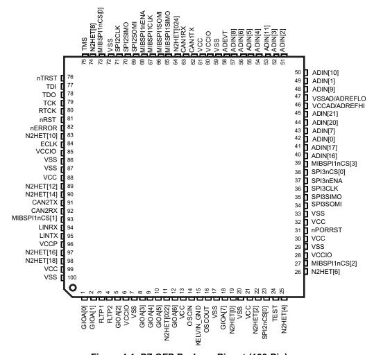
Figure 4-1. PZ QFP Package Pinout (100-Pin)
