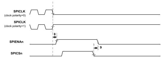
Figure 7-11. SPI Slave Mode Enable Timing (CLOCK PHASE = 0)
