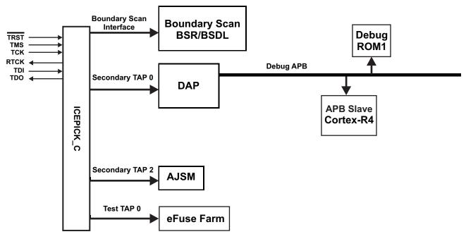
Figure 6-14. Debug Subsystem Block Diagram
