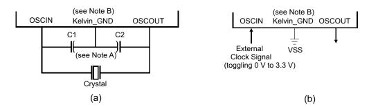
Note A: The values of C1 and C2 should be provided by the resonator/crystal vendor.
