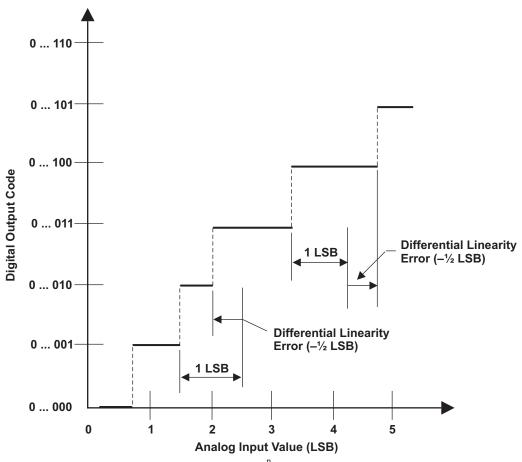
NOTE A:  $1 LSB = (AD_{REFHI} - AD_{REFLO})/2^n$  where n=10 in 10-bit mode and 12 in 12-bit mode
