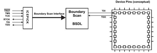
Figure 6-17. Boundary Scan Implementation (Conceptual Diagram)
