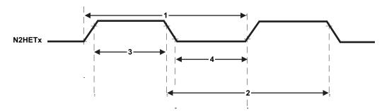
Figure 7-5. N2HET Input Capture Timings
