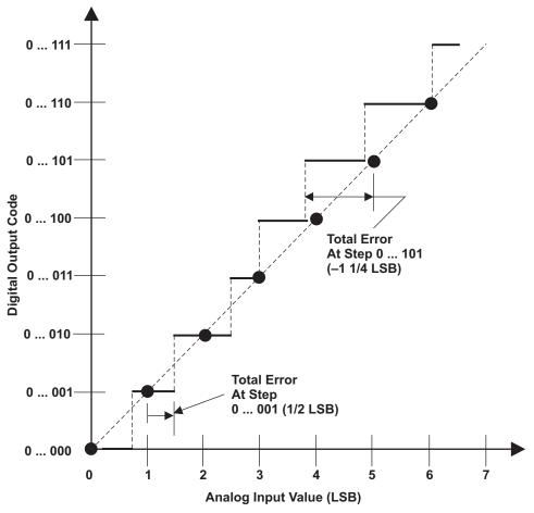
NOTE A:  $1 LSB = (AD_{REFHI} - AD_{REFLO})/2^n$  where n=10 in 10-bit mode and 12 in 12-bit mode
