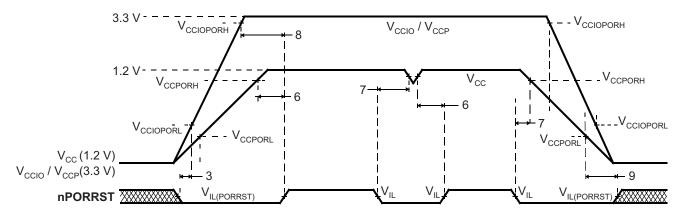
Note: There is no timing dependency between the ramp of the  $V_{\text{\tiny CCIO}}$  and the  $V_{\text{\tiny CCI}}$  supply voltage; this is just an example.
