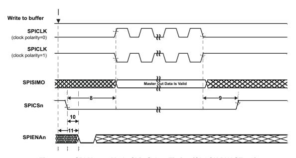
Figure 7-7. SPI Master Mode Chip Select Timing (CLOCK PHASE = 0)
