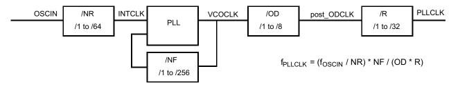
Figure 6-6. PLL Block Diagram
