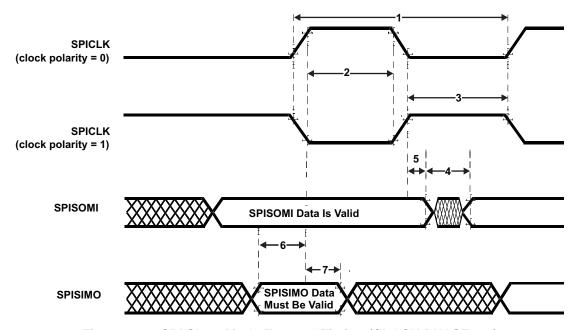
Figure 7-12. SPI Slave Mode External Timing (CLOCK PHASE = 1)
