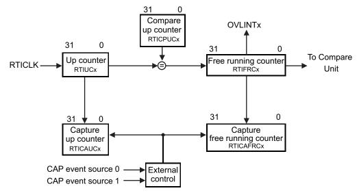
Figure 6-12. Counter Block Diagram
