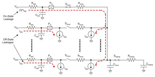
Figure 7-1. MibADC Input Equivalent Circuit
