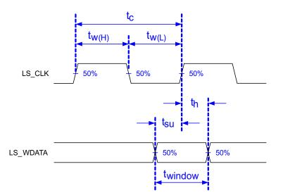
A. Low-speed interface is LPSDR and adheres to the *Electrical Characteristics* and AC/DC Operating Conditions table in JEDEC Standard No. 209B, *Low Power Double Data Rate (LPDDR)* JESD209B.
