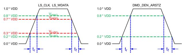
Figure 3. LPSDR Input Rise and Fall Slew Rate
