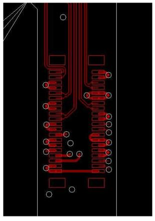
Figure 24. High-Speed (HS) Bus Connections
