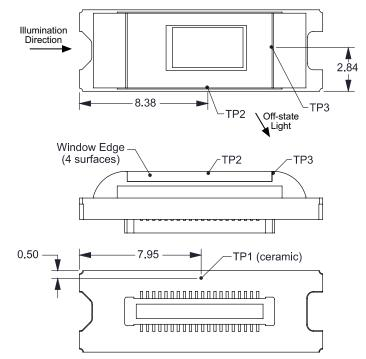
Figure 18. DMD Thermal Test Points
