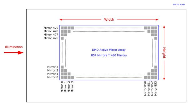
Figure 15. Micromirror Array Physical Characteristics
