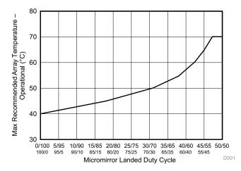
Figure 1. Maximum Recommended Array Temperature – Derating Curve
