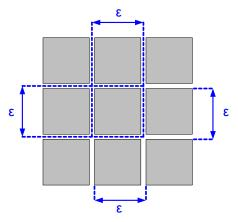
Figure 16. Mirror (Pixel) Pitch
