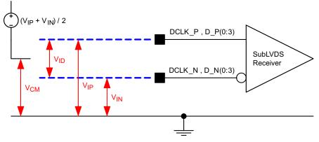
Figure 8. SubLVDS Voltage Parameters
