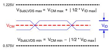
Figure 9. SubLVDS Waveform Parameters
