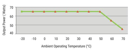
Output Power - Conection vs. Ambient Temperature
