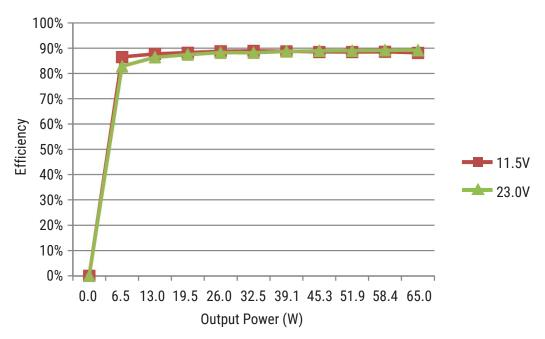
High efficiency is achieved by using QR technology. Synchronous MOSFETs or ultra-fast diodes are used as rectifiers in MB65S family.
