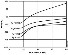
Figure 28. THD vs. Analog Input Frequency and Source Resistance
