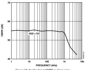
Figure 27. Analog Input CMRR vs. Frequency
