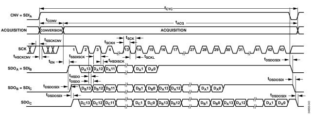
Figure 44. Chain Mode with BUSY Indicator Serial Interface Timing
