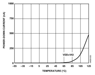
Figure 19. Power-Down Current vs. Temperature
