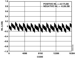
Figure 6. Integral Nonlinearity vs. Code
