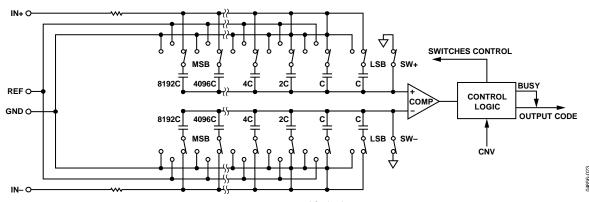
Figure 23. ADC Simplified Schematic
