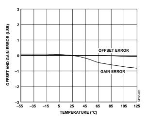
Figure 21. Offset and Gain Error vs. Temperature
