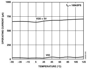
Figure 20. Operating Current vs. Temperature
