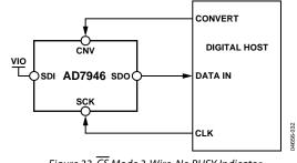
Figure 33. CS Mode 3-Wire, No BUSY Indicator Connection Diagram (SDI High)
