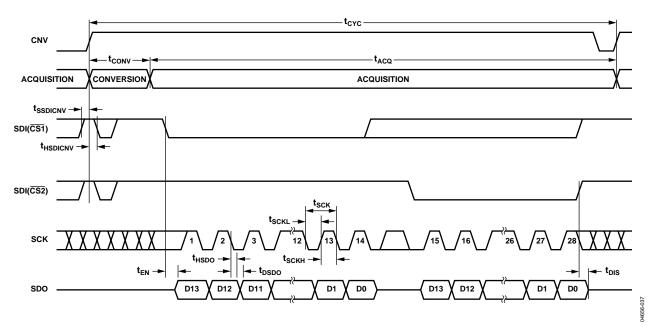
Figure 38. CS Mode 4-Wire, No BUSY Indicator Serial Interface Timing
