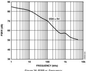
Figure 29. PSRR vs. Frequency
