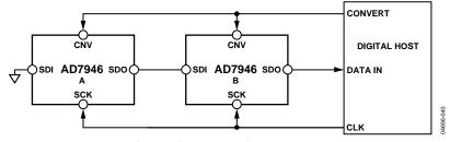
Figure 41. Chain Mode, No BUSY Indicator Connection Diagram
