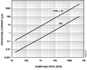
Figure 30. Operating Currents vs. Sampling Rate
