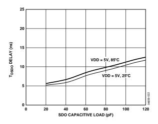
Figure 22. t<sub>DSDO</sub> Delay vs. Capacitance Load and Supply
