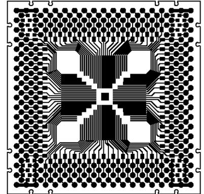
Support up to 100 pins QFP, TQFP, PQFP package IC with .5mm Pitch; 20 pcs. of 0603 package, and some thru hole passive components. 6 ground holes are connected a copper plane on the bottom side. A hole in the center gives access to a ground or thermal pad on IC.
