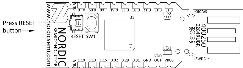
When the nRF52840 Dongle has entered the bootloader mode, **LD2** pulses red. The Dongle is now ready for programming.
