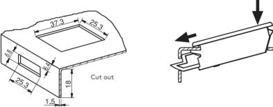
Follow the arrows for assembly instructions; open or close with internal movable parts
