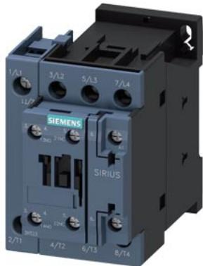
Contactor, AC-1, 35 A/400 V/40 °C, S0, 4-pole, 220 V AC/50 Hz, 240 V/60 Hz, 1 NO+1 NC, screw terminal
