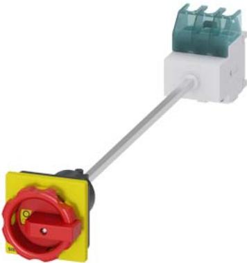
SENTRON, Switch disconnector 3LD, emergency switching-off switch, 3-pole,  $I_{u}$ : 25 A, operating power / at AC-23 A 400 V: 9.5 kW, floor mounting with door coupling, rotary operating mechanism, Red / yellow, 4-hole mounting of the handle
