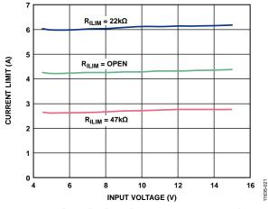
Figure 23. Channel 1/Channel 2 Current Limit vs. Input Voltage
