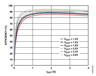
Figure 5. Channel 1/Channel 2 Efficiency Curve,  $V_{IN} = 12 V$ ,  $f_{SW} = 600 \text{ kHz}$ , FPWM Mode
