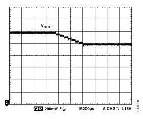
Figure 35. Channel 1 Dynamic Voltage Scaling (DVS) from 1.3 V to 1.1 V, 62.5 µs Interval,  $V_{IN} = 12$  V,  $I_{OUT} = 4$  A,  $f_{SW} = 600$  kHz, L = 1 µH,  $C_{OUT} = 47$  µF  $\times 2$
