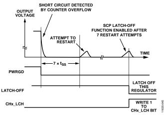
Figure 47. Short-Circuit Latch-Off Detection
