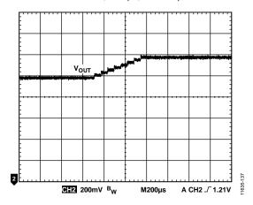
Figure 34. Channel 1 Dynamic Voltage Scaling (DVS) from 1.1 V to 1.3 V, 62.5 µs Interval,  $V_{IN} = 12$  V,  $I_{OUT} = 4$  A,  $f_{SW} = 600$  kHz, L = 1 µH,  $C_{OUT} = 47$  µF  $\times 2$
