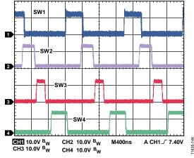
Figure 41. I<sup>2</sup>C Configurable 90° Phase Shift Waveforms, Four Buck Regulators
