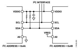
Figure 56. Two ADP5051 Devices Configured with Different I<sup>2</sup>C Addresses (A0 Function Replaces PWRGD Function on Pin 20)
