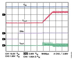
Figure 30. Startup with Precharged Output,  $V_{IN} = 12 V$ ,  $V_{OUT} = 3.3 V$
