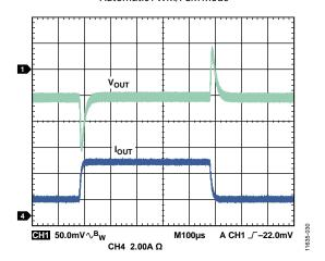
Figure 27. Channel 1/Channel 2 Load Transient, 1 A to 4 A,  $V_{IN} = 12$  V,  $V_{OUT} = 3.3$  V,  $f_{SW} = 600$  kHz, L = 2.2 µH,  $C_{OUT} = 47$  µF  $\times 2$
