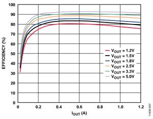
Figure 9. Channel 3/Channel 4 Efficiency Curve,  $V_{IN} = 12 V$ ,  $f_{SW} = 600 \text{ kHz}$ , FPWM Mode
