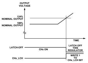
Figure 48. Overvoltage Latch-Off Detection
