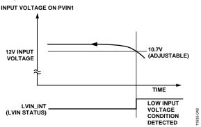
Figure 50. Low Input Voltage Warning Function ( $V_{IN} = 12 V$ )
