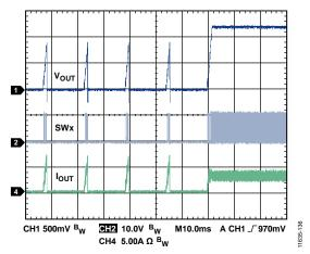
Figure 33. Short-Circuit Protection Recovery,  $V_{IN} = 12 V$ ,  $V_{OUT} = 1.2 V$ ,  $f_{SW} = 600 \text{ kHz}$ ,  $L = 1 \mu$ H,  $C_{OUT} = 47 \mu$ F  $\times 2$
