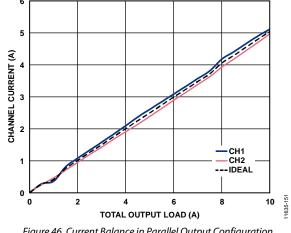
Figure 46. Current Balance in Parallel Output Configuration,  $V_{IN} = 12 V$ ,  $V_{OUT} = 1.2 V$ ,  $f_{SW} = 600 \text{ kHz}$ , FPWM Mode
