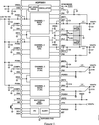
Combining Channel 1 and Channel 2 in a parallel configuration provides a single output with up to 8 A of current. Channel 3 and Channel 4 integrate both high-side and low-side MOSFETs to deliver an output current of 1.2 A.
