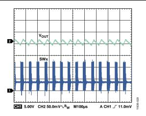
Figure 26. Steady State Waveform at Light Load,  $V_{IN} = 12 V$ ,  $V_{OUT} = 3.3 V$ ,  $I_{OUT} = 30 \text{ mA}$ ,  $f_{SW} = 600 \text{ kHz}$ ,  $L = 4.7 \mu\text{H}$ ,  $C_{OUT} = 47 \mu\text{F} \times 2$ , Automatic PWM/PSM Mode
