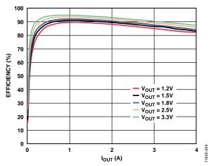
Figure 6. Channel 1/Channel 2 Efficiency Curve,  $V_{IN} = 5.0 V$ ,  $f_{SW} = 600 kHz$ , FPWM Mode
