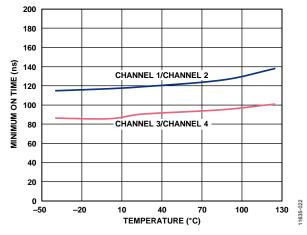
Figure 24. Minimum On Time vs. Temperature
