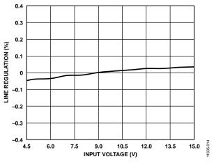
Figure 16. Channel 3 Line Regulation,  $V_{OUT} = 3.3 V$ ,  $I_{OUT} = 1 A$ ,  $f_{SW} = 600 \text{ kHz}$ , FPWM Mode
