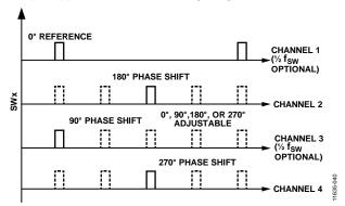
Figure 40. Phase Shift Diagram, Four Buck Regulators
