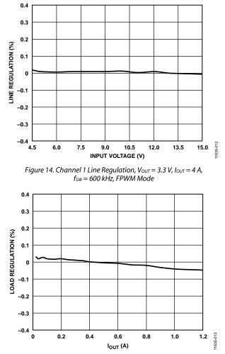
Figure 15. Channel 3 Load Regulation,  $V_{IN} = 12$  V,  $V_{OUT} = 3.3$  V,  $f_{SW} = 600$  kHz, FPWM Mode
