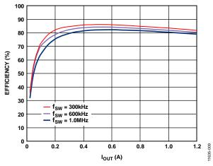
Figure 11. Channel 3/Channel 4 Efficiency Curve,  $V_{IN} = 12 V$ ,  $V_{OUT} = 1.8 V$ , FPWM Mode
