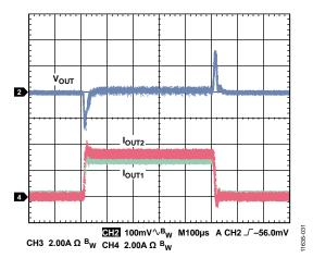
Figure 28. Load Transient, Channel 1/Channel 2 Parallel Output, 0 A to 6 A,  $V_{IN} = 12 V$ ,  $V_{OUT} = 3.3 V$ ,  $f_{SW} = 600 \text{ kHz}$ ,  $L = 4.7 \mu\text{H}$ ,  $C_{OUT} = 47 \mu\text{F} \times 4$
