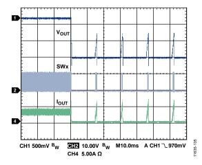
Figure 32. Short-Circuit Protection Entry,  $V_{IN} = 12 V$ ,  $V_{OUT} = 1.2 V$ ,  $f_{SW} = 600 \text{ kHz}$ ,  $L = 1 \mu$ H,  $C_{OUT} = 47 \mu$ F  $\times 2$
