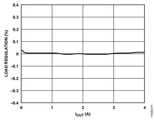
Figure 13. Channel 1 Load Regulation,  $V_{IN} = 12 V$ ,  $V_{OUT} = 3.3 V$ ,  $f_{SW} = 600 kHz$ , FPWM Mode
