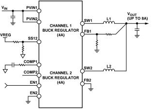
Figure 45. Parallel Operation for Channel 1 and Channel 2
