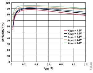
Figure 10. Channel 3/Channel 4 Efficiency Curve,  $V_{IN} = 5.0 V$ ,  $f_{SW} = 600 kHz$ , FPWM Mode
