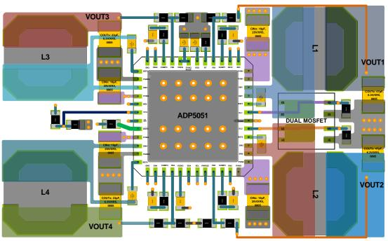
Figure 63. Typical PCB Layout
