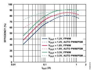
Figure 12. Channel 3/Channel 4 Efficiency Curve,  $V_{IN} = 12 V$ ,  $f_{SW} = 600 kHz$ , FPWM and and Automatic PWM/PSM Modes
