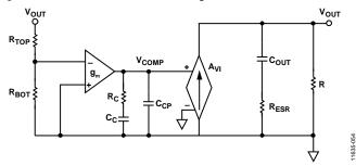
Figure 59. Simplified Peak Current Mode Control Small Signal Circuit
