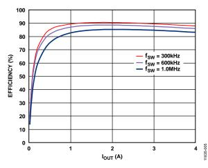
Figure 7. Channel 1/Channel 2 Efficiency Curve,  $V_{IN} = 12 V$ ,  $V_{OUT} = 1.8 V$ , FPWM Mode
