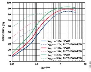
Figure 8. Channel 1/Channel 2 Efficiency Curve,  $V_{IN} = 12 V$ ,  $f_{SW} = 600 \text{ kHz}$ , FPWM and Automatic PWM/PSM Modes
