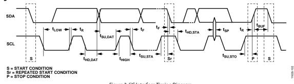
Figure 3. I<sup>2</sup>C Interface Timing Diagram
