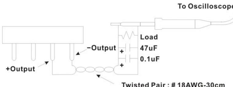
A 30cm twisted pair of no.18 AWG copper wire is connected to a 47uF and 0.1uF capacitor of proper polarity and voltage rating. The oscilloscope probe ground lead should connect right to the ground ring of the probe and be as short as possible. The oscilloscope bandwidth should be at 20MHz and connected to AC ground.
