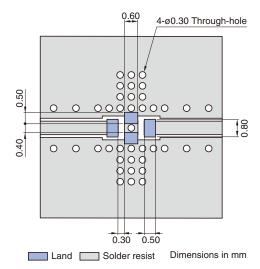
Line width be designed to match  $50\Omega$ characteristic impedance depending on PCB material and thickness.
