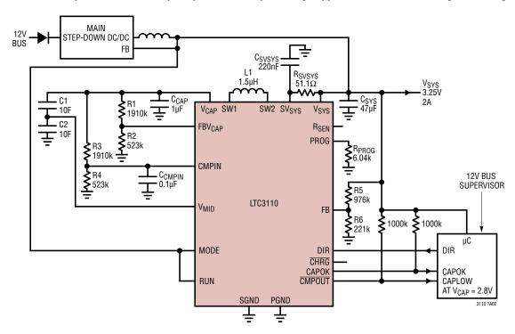
1.8V/300mA Output from Single Capacitor Discharged from 2.5V to 1V and with Reserve Available Down to 0.3V
