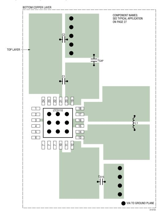
Figure 20. PCB Component Placement of the QFN Package
