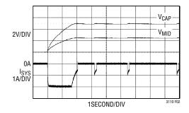
Figure 2. Charge Foldback and Charge Termination
