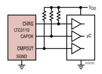
Figure 18. Outputs  $\overline{\text{CHRG}}$ , CAPOK,  $\overline{\text{CMPOUT}}$  Interfacing to  $\mu\text{C}$
