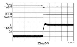
Figure 1. Transition from Charge<sup>-</sup> into Backup Operation
