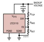
Figure 11. Voltage with Reduced Tolerances
