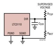
Figure 12. Filtering DIR voltage
