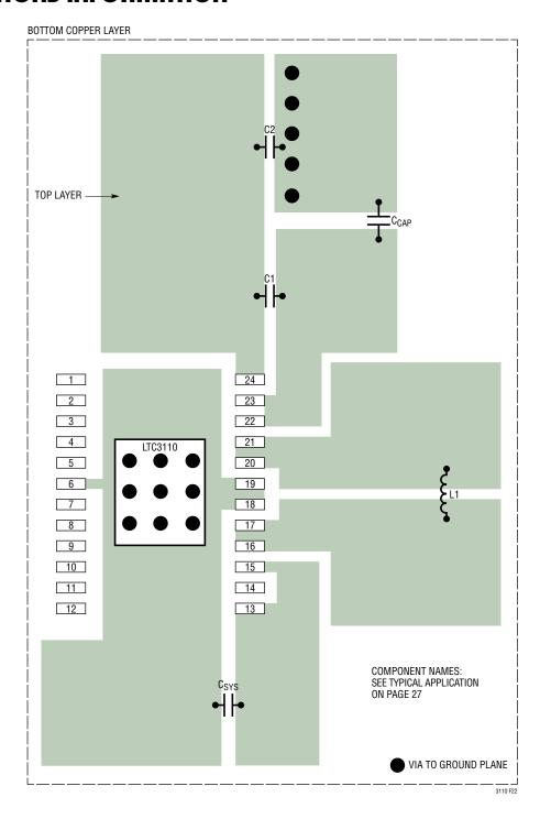
Figure 19. PCB Component Placement of the TSSOP Package
