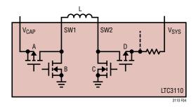
Figure 4. Buck-Boost Switch Topology
