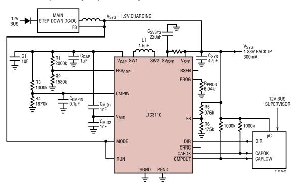
500mA USB Charge/Backup Application with Variable Charging Power, P<sub>CHRG</sub>, Depending on System Load
