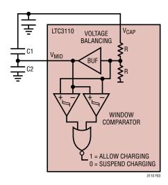
Figure 3. Active Charge Balancer
