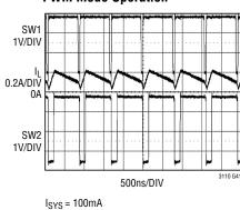
PWM Mode Operation in V<sub>CAP</sub> Overvoltage Failure Condition
