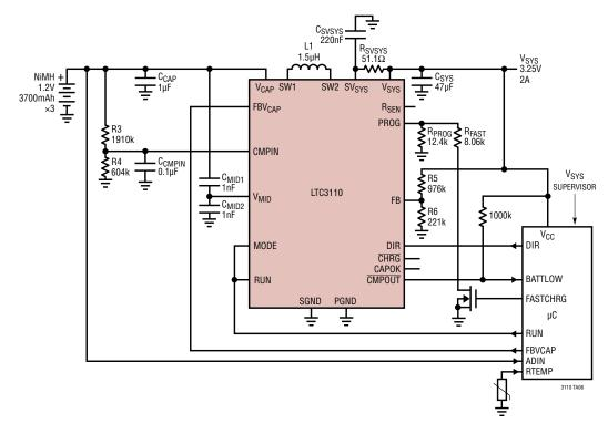
NOTE ON DIGITAL CONTROL SIGNALS IN NIMH BACKUP/RECHARGE APPLICATION: CHARGING IS INITIATED BY PULLING DIR = HIGH AND  $FBV_{CAP} = LOW$ . CHARGING IS TERMINATED BY PULLING DIR = HIGH AND  $FBV_{CAP} = HIGH$  ( $FBV_{CAP}$  MUST  $BE \geq 1.2V$ ). SYSTEM BACK-UP IS INITIATED BY FORCING FBVCAP = LOW, WAITING  $5\mu s$ , THEN FORCING DIR = LOW.
