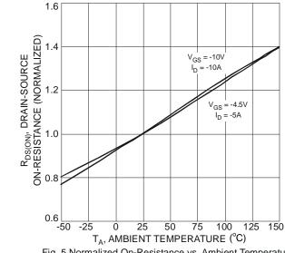
Fig. 5 Normalized On-Resistance vs. Ambient Temperature
