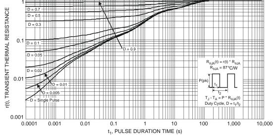
Fig. 11 Transient Thermal Response
