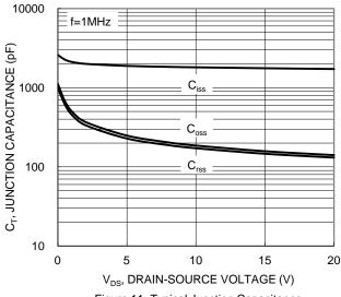
Figure 11. Typical Junction Capacitance
