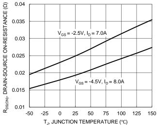
Figure 7. On-Resistance Variation with Junction Temperature
