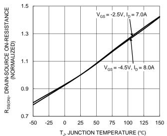
Figure 6. On-Resistance Variation with Junction Temperature
