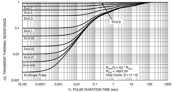
Figure 14. Transient Thermal Resistance
