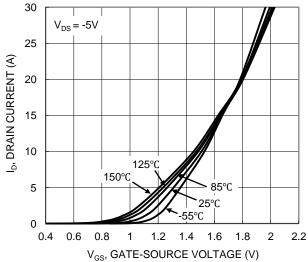
Figure 2. Typical Transfer Characteristic
