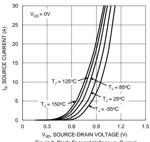
Figure 9. Diode Forward Voltage vs. Current
