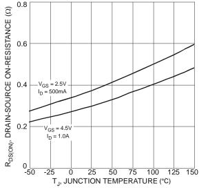
Figure 6 On-Resistance Variation with Temperature
