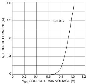
Figure 8 Diode Forward Voltage vs. Current
