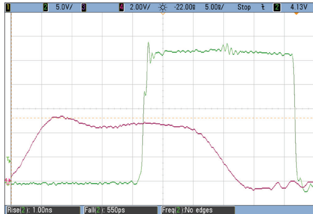
Figure 4: Typical Waveforms for V_{IN} = 28V to 3.3V/4A (5 MHz) Buck converter CH2: ( V_{OUT} ) Switch node voltage — CH4: V_{PWM} Input voltage
