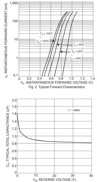
Fig. 4 Typical Capacitance vs. Reverse Voltage
