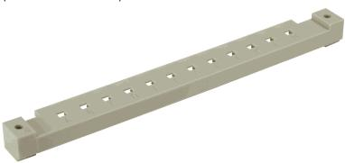
This coding system is an integral part of both male and female connectors. A comb with 12 coding pins, which is supplied under part number 09 02 000 9928, allows over 900 coding variations. The pins are to be locked into the male and female connectors.
