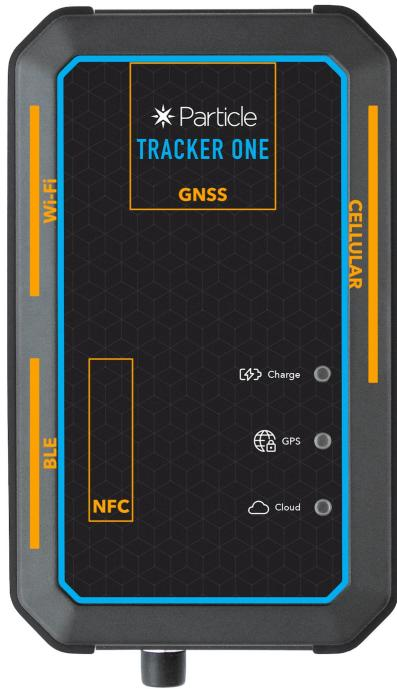
As the GNSS antenna faces the top of the case, you also want the top of the case facing the sky to the greatest extent possible. You will likely be unable to get a GNSS lock with the top facing down.
