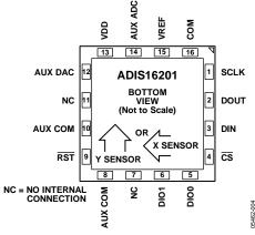
Figure 4. Pin Configuration
