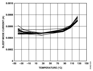
Figure 29. Sleep Mode Current vs. Temperature at 3.3 V
