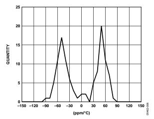
Figure 6. Acceleration Sensitivity Tempco Histogram at 3.3 V
