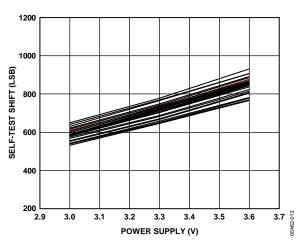
Figure 13. Self-Test Shift vs. Supply at 25  $^{\circ}$ C
