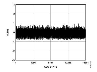
Figure 20. Typical ADC Differential Nonlinearity
