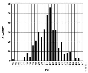
Figure 25. Temperature Distribution at 25°C/3.3 V
