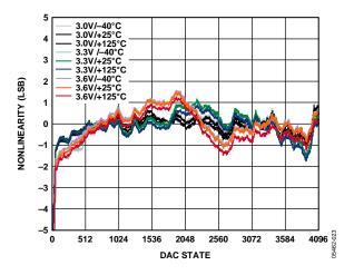
Figure 23. Typical DAC Integral Nonlinearity
