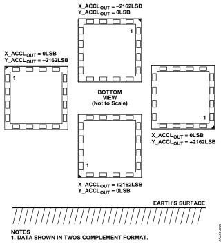
Figure 36. Output Response vs. Orientation
