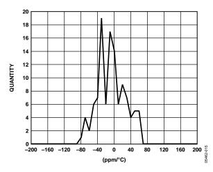
Figure 15. Inclination Offset Tempco Histogram at 3.3 V
