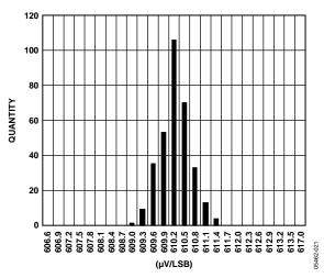
Figure 21. DAC Gain Distribution at 25°C/3.3 V
