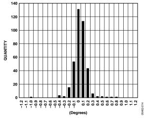
Figure 14. Inclination Offset Distribution at 25°C/3.3 V/0 g
