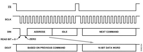
Figure 31. Register Read Command Sequence
