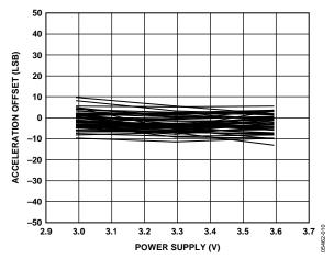
Figure 10. Acceleration Offset vs. Supply at 25°C
