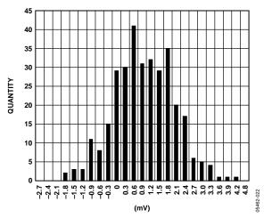
Figure 22. DAC Offset Distribution at 25°C/3.3 V
