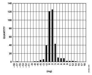
Figure 8. Acceleration Offset Distribution at 25°C/3.3 V/0 g
