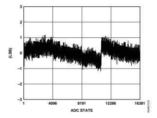
Figure 19. Typical ADC Integral Nonlinearity at 25°C/3.3 V
