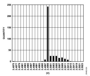
Figure 24. VREF Distribution at 25°C/3.3 V
