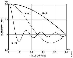
Figure 34. Number of Taps vs. Sample Frequency Response
