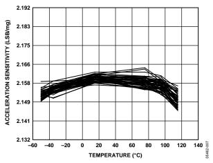
Figure 7. Acceleration Sensitivity vs. Temperature at 3.3 V
