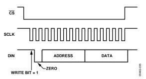
Figure 32. Control Register Write Command Sequence of SPI Signals
