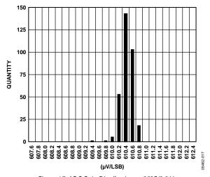
Figure 17. ADC Gain Distribution at 25°C/3.3 V
