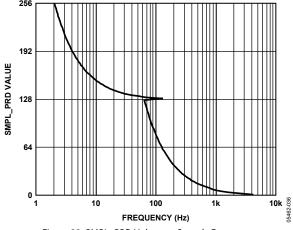
Figure 33. SMPL\_PRD Values vs. Sample Frequency
