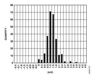
Figure 18. ADC Offset Distribution at 25°C/3.3 V
