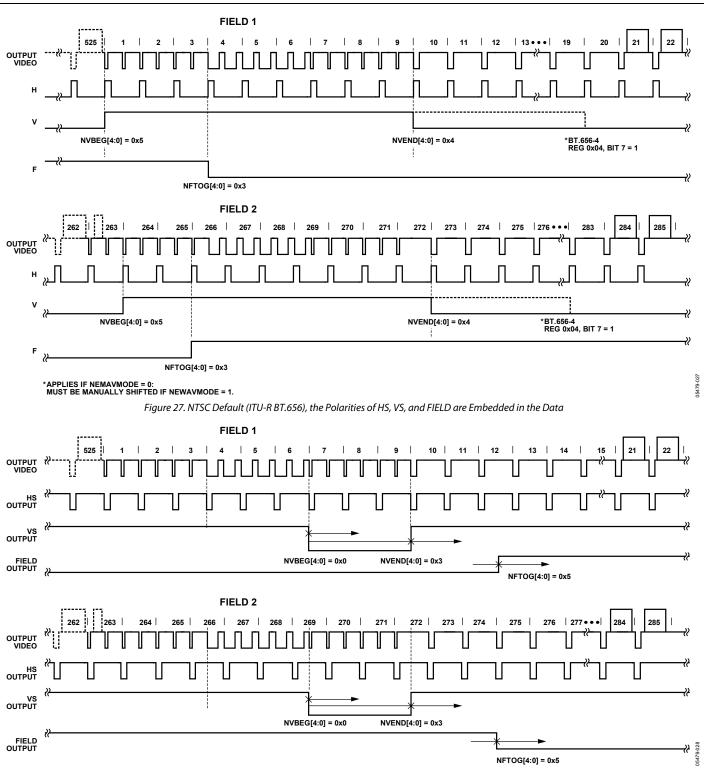
Figure 28. NTSC Typical VS/FIELD Positions Using Register Writes in Table 62
