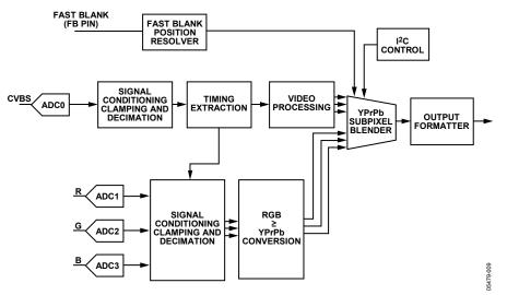
Figure 9. Fast Blanking Configuration
