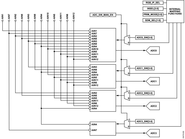
Figure 6. Internal Pin Connections
