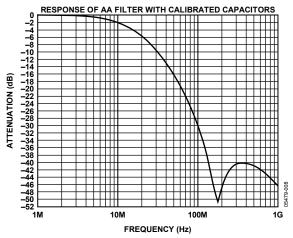
Figure 8. Frequency Response of Internal ADV7184 Antialiasing Filters
