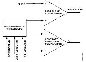
Figure 11. Fast Blank and Contrast Reduction Programmable Threshold
