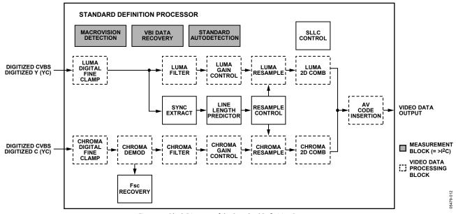
Figure 12. Block Diagram of the Standard Definition Processor
