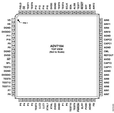
Figure 5. 80-Lead LQFP Pin Configuration
