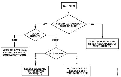
Figure 15. YSFM and WYSFM Control Flowchart
