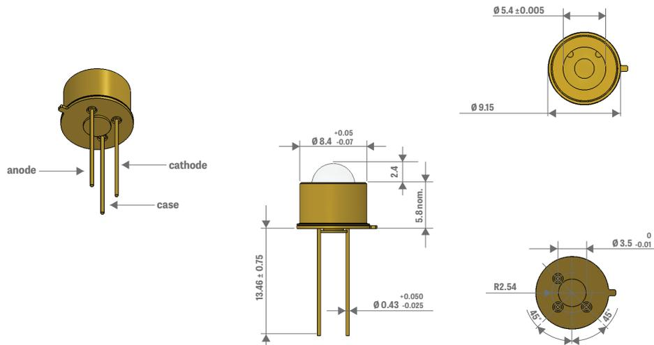
All dimensions are in millimeters. Unless noted otherwise, all dimensions have a tolerance of ± 0.05 mm.
