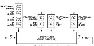
Figure 42. Third Order Digital IIR Loop Filter
