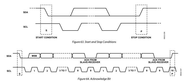
The acknowledge bit (A) is the ninth bit attached to any 8-bit data byte. An acknowledge bit is always generated by the receiving device (receiver) to inform the transmitter that the byte has been received. It is done by pulling the SDA line low during the ninth clock pulse after each 8-bit data byte.
