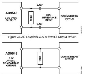
Figure 29. DC-Coupled LVDS or LVPECL Output Driver
