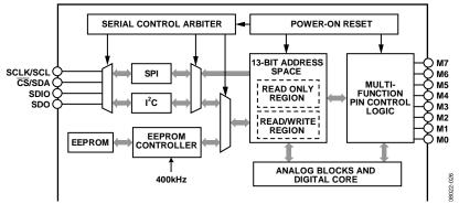
Figure 53. Serial Port Functional Diagram
