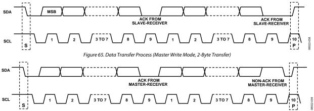
Figure 66. Data Transfer Process (Master Read Mode, 2-Byte Transfer)
