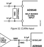
Figure 33. System Clock Input (SYSCLKP/SYSCLKN) When Using a TCXO/OCXO with 3.3 V CMOS Output
