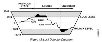
Note that whenever the AD9548 enters the free-run or holdover mode, the DPLL phase lock detector indicates unlocked. In addition, whenever the AD9548 performs a reference switchover, the state of the lock detector prior to the switch is preserved during the transition period.
