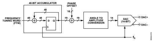
Figure 44. DDS Block Diagram
