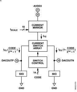
Figure 45. DAC Output Pins
