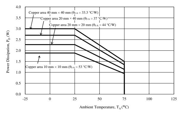
Figure 6-1. Power Dissipation, P<sub>D</sub> vs. Ambient Temperature, T<sub>A</sub>
