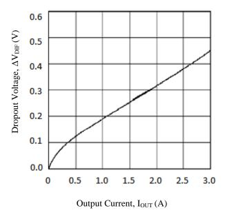
Figure 5-1. Dropout Voltage
