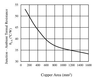
Figure 13-3 Thermal Resistance – Copper Area Reference Characteristics (Single-sided Copper Foil Board, FR-4)
