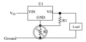
Figure 13-2 Output Voltage Setting (Do not connect R2.)
