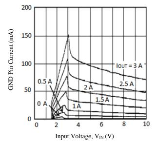
Figure 5-3. GND Pin Current
