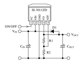
Figure 9-1. Typical Application ( $V_{OUT} > 1.8 \text{ V}$ )
