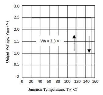
Figure 5-9. Thermal Shutdown Characteristics
