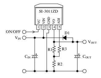
Figure 9-2. Typical Application ( $V_{OUT} \le 1.8 \text{ V}$ )
