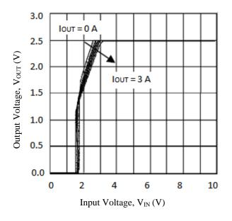
Figure 5-2. Output Rise Characteristics
