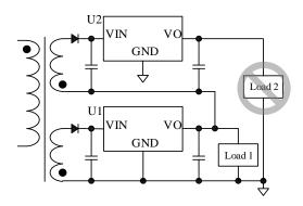
Figure 13-1 Stacked on Loads (Do not connect Load 2.)
