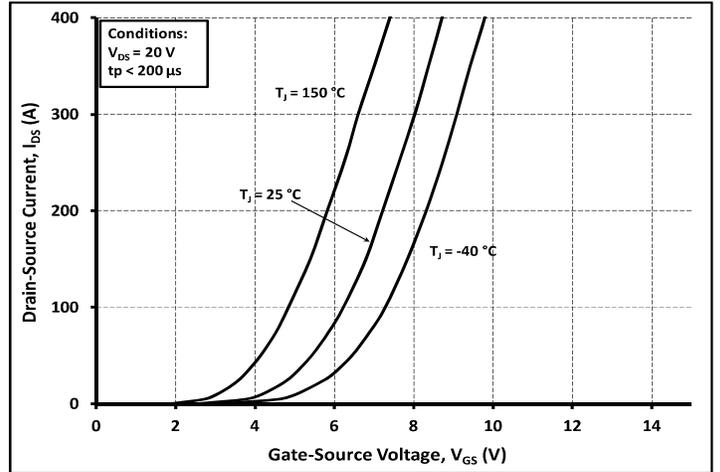
Figure 8. Transfer Characteristic for Various Junction Temperatures
