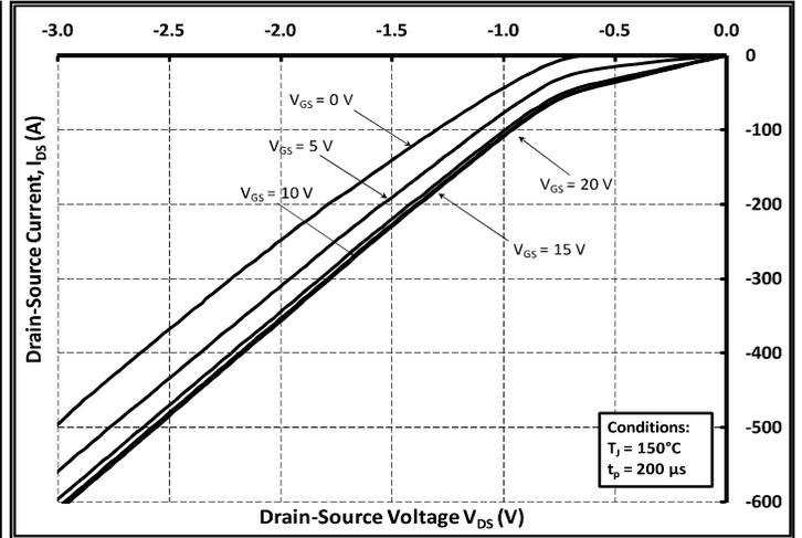
Figure 14. 3<sup>rd</sup> Quadrant Characteristic at 150 °C
