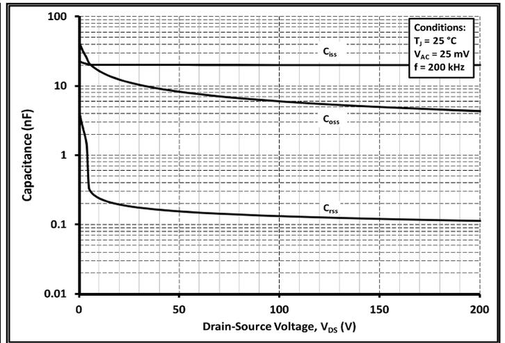
Figure 16. Capacitances vs. Drain-Source Voltage (0 - 200 V)
