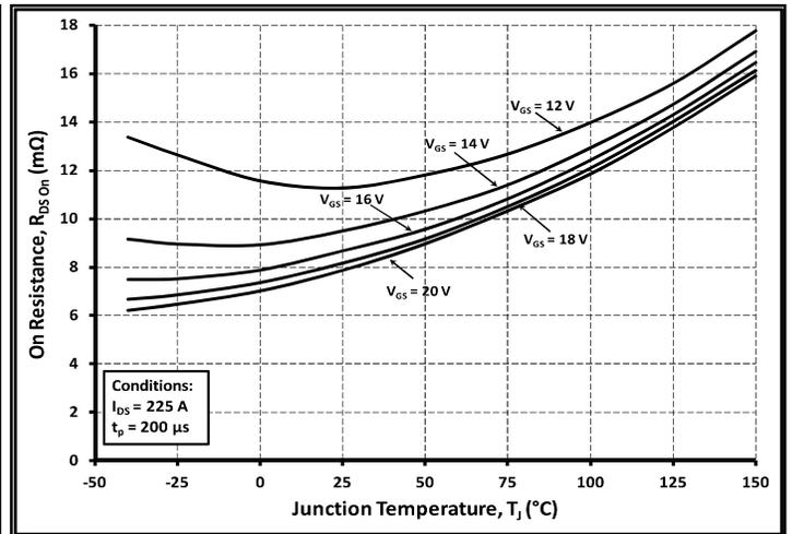
Figure 6. On-Resistance vs. Temperature for Various Gate-Source Voltage
