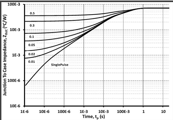
Figure 27. MOSFET Junction to Case Thermal Impedance
