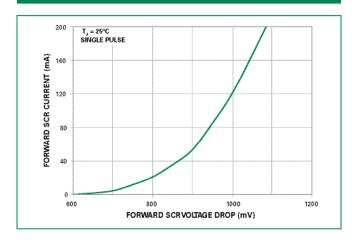
Figure 3: High Current SCR Forward Voltage Drop Curve
