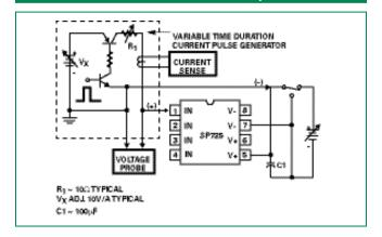
Figure 5: SP725 Typical Nonrepetitive Peak Current **Pulse Capability**
