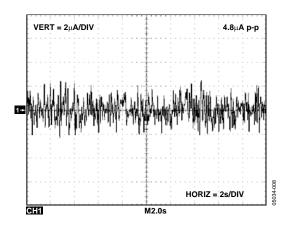
Figure 9. 0.1 Hz to 10 Hz Noise Plot (VDD = 3.6 V)
