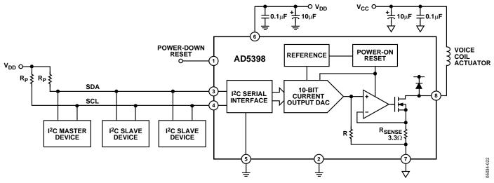
Figure 22. Typical Application Circuit
