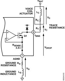
Figure 20. Effect of PCB Trace Resistance and Inductance
