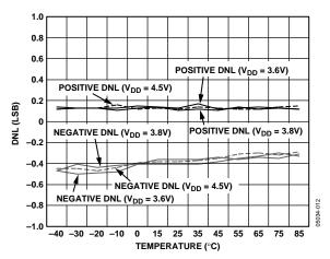
Figure 13. DNL vs. Temperature vs. Supply
