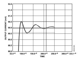
Figure 7. ¼ to ¾ Scale Settling Time (VDD = 3.6 V)
