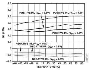
Figure 12. INL vs. Temperature vs. Supply
