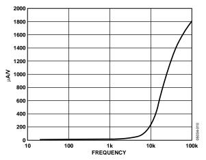
Figure 11. AC Power Supply Rejection (VDD = 3.6 V)
