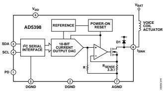
Figure 16. Block Diagram Showing Connection to Voice Coil
