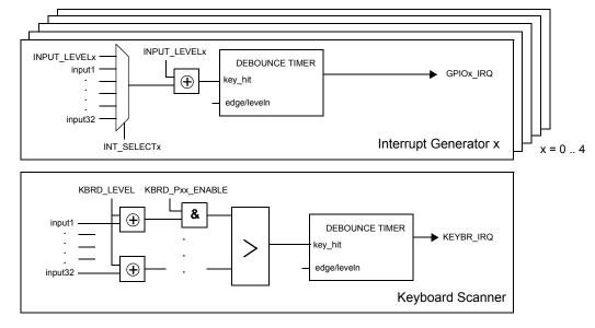
Figure 51: Keyboard Controller Block Diagram
