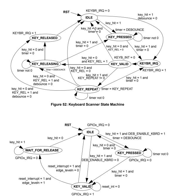
Figure 53: GPIO Interrupt Generator State Machine
