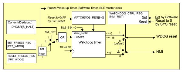
Figure 50: Watchdog Timer Block Diagram
