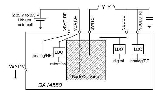
Figure 57: Supply Overview, Coin-Cell Application
