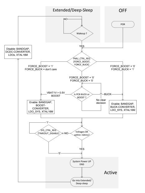
Figure 7: Power/Wake-Up Sequence
