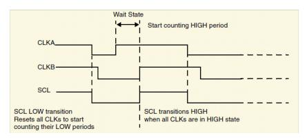
Figure 29: Multiple Master Clock Synchronization
