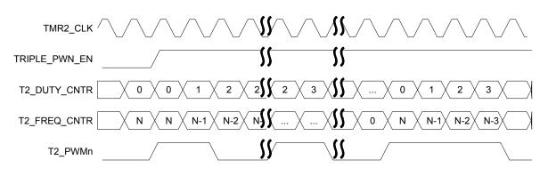
Figure 49: Timer 2 PWM Timing Diagram
