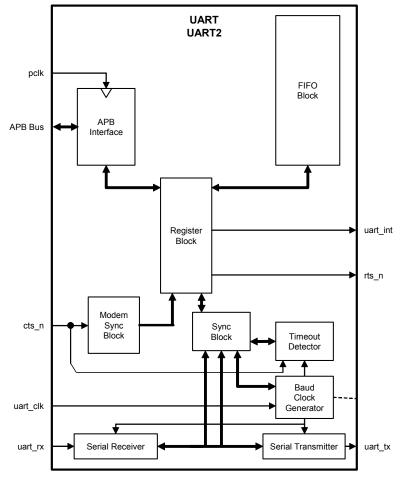
Figure 30: UART Block Diagram
