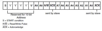
Figure 24: 10-bit Address Format
