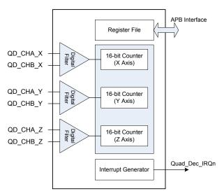
Figure 41: Quadrature Decoder Block Diagram
