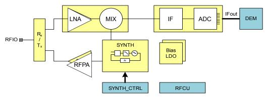
Figure 67: Bluetooth Radio Block Diagram
