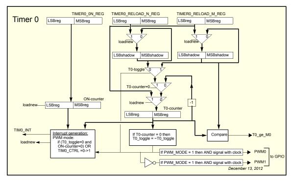
Figure 46: Timer 0 Block Diagram
