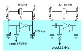
Figure 15: Crystal Oscillator Circuits
