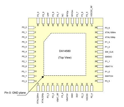
Figure 3: QFN48 Pin Assignment
