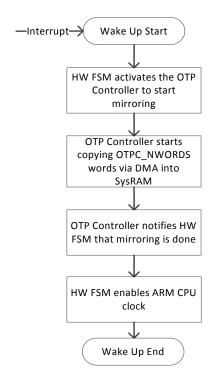
Figure 8: Wake-Up OTP Mirroring
