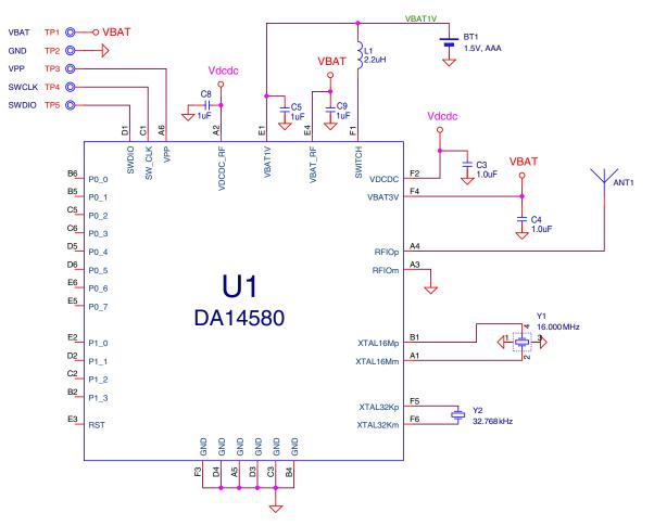
Figure 68: Alkaline Battery Cell Powered System Diagram (Boost Mode)
