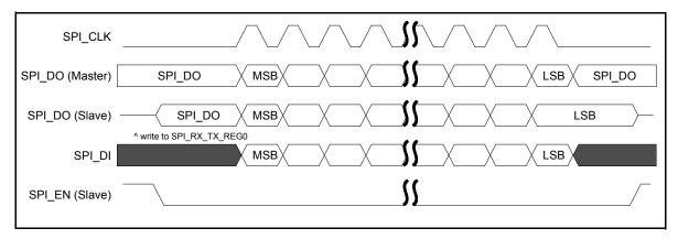
Figure 38: SPI Master/Slave, Mode 1: SPI\_POL=0 and SPI\_PHA=1
