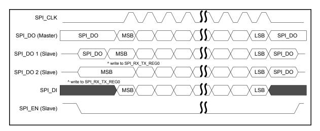
Figure 37: SPI Master/Slave, Mode 0: SPI\_POL=0 and SPI\_PHA=0
