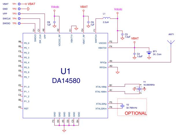
Figure 69: Lithium Coin Cell Powered System Diagram (Buck Mode)
