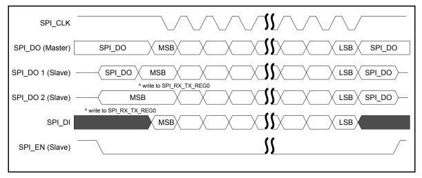
Figure 39: SPI Master/Slave, Mode 2: SPI\_POL=1 and SPI\_PHA=0
