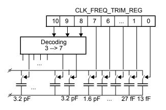
Figure 16: Frequency Trimming
