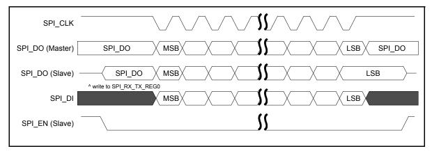
Figure 40: SPI Master/Slave, Mode 3: SPI\_POL=1 and SPI\_PHA=1
