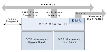
Figure 18: OTP Controller Block Diagram
