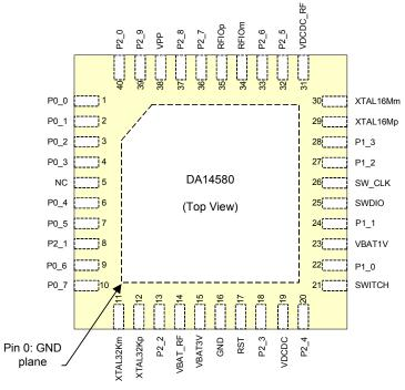
Figure 4: QFN40 Pin Assignment
