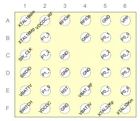
Figure 2: WLCSP34 ball assignment
