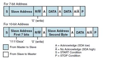
Figure 25: Master-Transmitter Protocol
