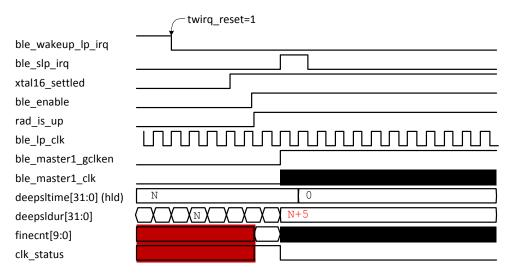
Figure 64 Exit BLE Deep Sleep Mode Later Than the Predetermined Time (Zoom In)
