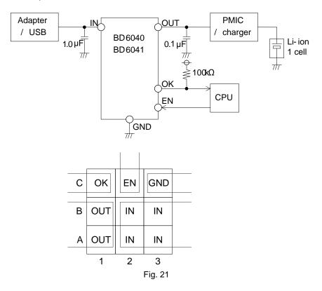
B: In case of OK pin is connected.
