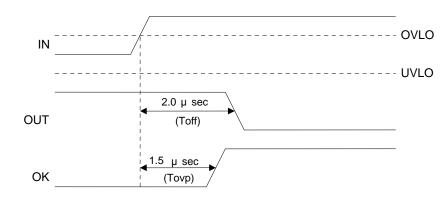
Fig. 19 Shutdown by over voltage detection
