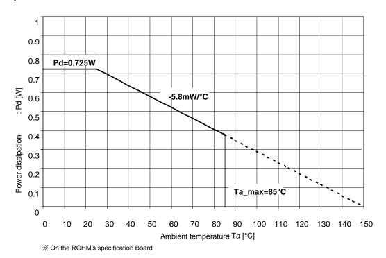
Fig. 25 Power dissipation vs. Ta
