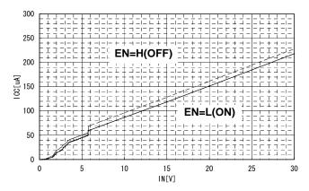
Fig. 7 ICC vs. Input Voltage (0-30V)
