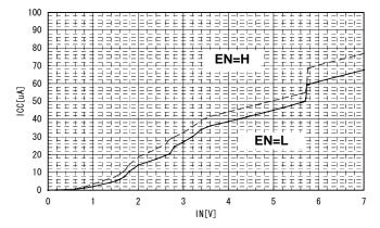
Fig. 8 ICC vs. Input Voltage (0-7V)
