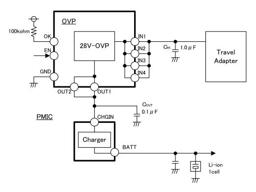
Fig. 17 Application Circuit
