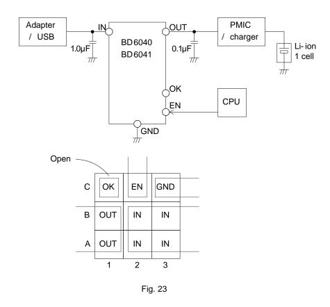
D: In case of both EN & OK pins are not connected.
