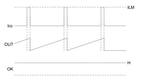
Fig. 20 Operation by current limit detection
