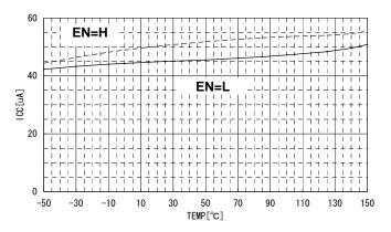
Fig. 9 ICC vs. Temperature (IN=5V)
