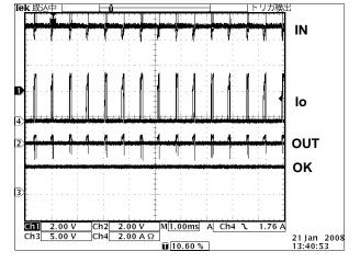
Fig. 5 Output Short Circuit
