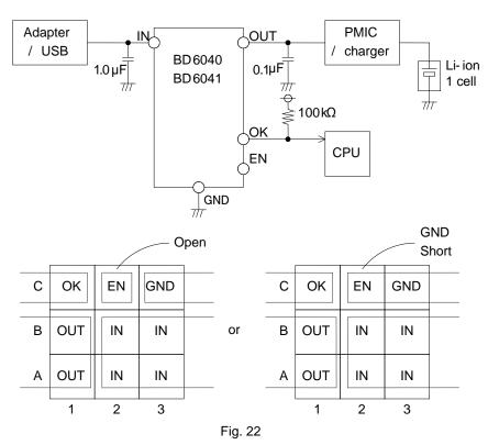
C: In case of EN pin is connected.
