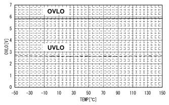
Fig. 10 UVLO/OVLO vs. Temperature
