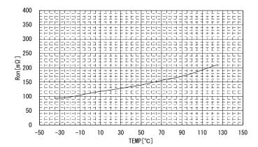
Fig. 12 RON vs. Temperature (IN=5V)
