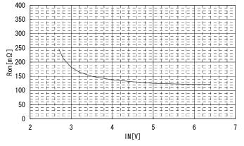
Fig. 11 RON vs. Input Voltage
