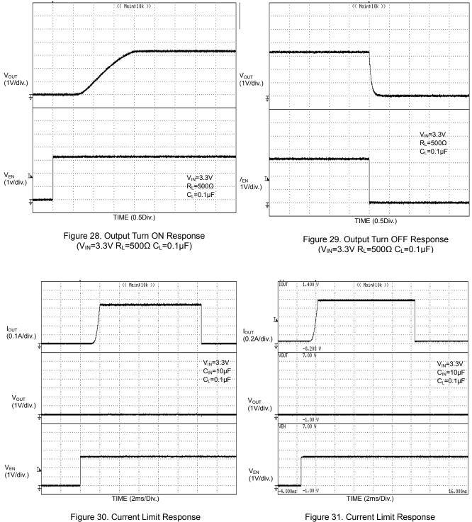
Enable Into Short Circuit ( $V_{IN}$ =3.3V C<sub>IN</sub>=10µF C<sub>L</sub>=0.1µF BD2202G)
