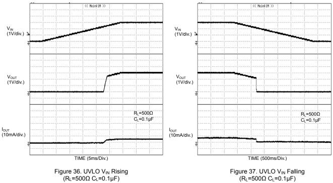
Figure 37. UVLO  $V_{IN}$  Falling (RL=500 $\Omega$  CL=0.1 $\mu F)$
