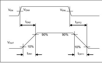
Figure 2. Switch Turn ON / OFF Time
