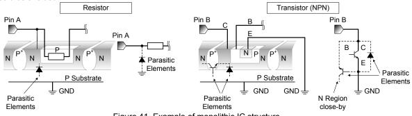
Figure 41. Example of monolithic IC structure
