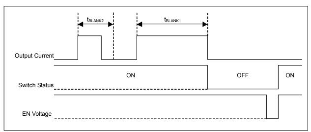
Figure 38. Over-Current Detection, Shutdown Operation (Return with EN Input)
