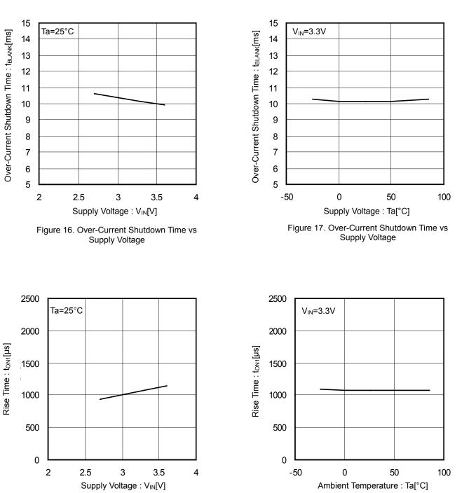
Figure 18. Output Rise Time vs Supply Voltage
