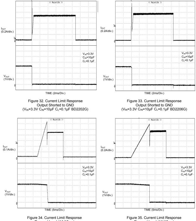
Ramped Load (1A/10ms) (V<sub>IN</sub>=3.3V C<sub>IN</sub>=10µF C<sub>L</sub>=0.1µF BD2202G)
