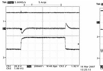
Figure 3- Step load 1.2-2.8A, ch1: Vin ch2: Vout, ch3: lout
