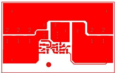
Figure 11. SP6125EB PCB Layout Top Side
