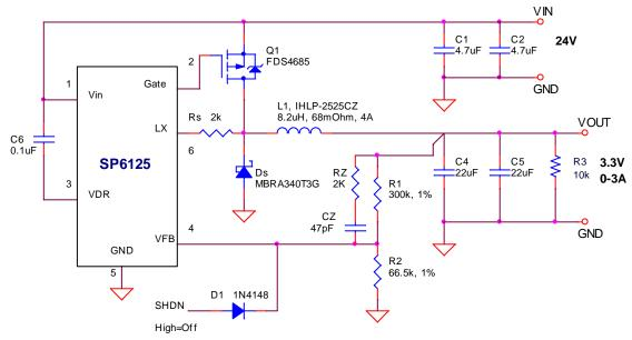
\* R(10k) is optional. It helps keep the output capacitor discharged under no-load condition.
