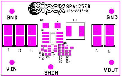
Figure 10. SP6125EB Component Placement
