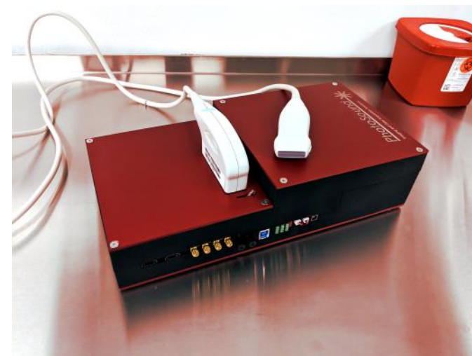
PhotoSound® MoleculUS™, ultrasonic imaging with molecular analysis
