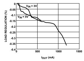
FIGURE 4. VBOOST LOAD REGULATION (PI MODE)
