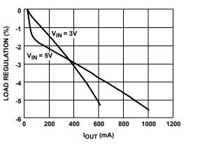
FIGURE 5. VBOOST LOAD REGULATION (P MODE)
