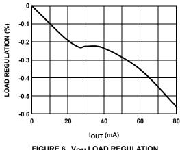
FIGURE 6. VON LOAD REGULATION
