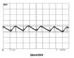
FIGURE 19. VBOOST OUTPUT VOLTAGE RIPPLE
