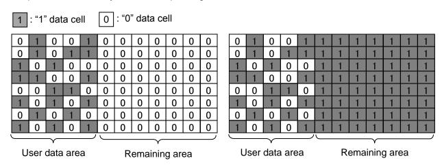
(a) Accelerate block endurance degradation by fixed dummy "0" data write
