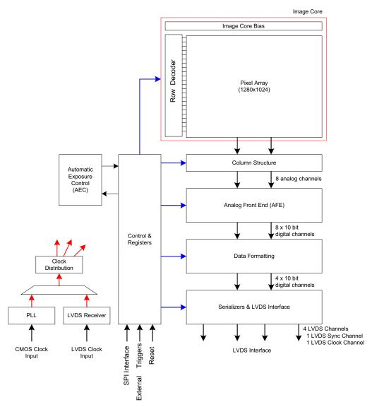
Figure 4. Block Diagram - V1-SN/SE
