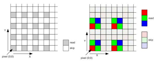
Figure 24. Subsampling Scheme for Monochrome and Color Sensors
