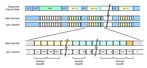
Figure 32. V1-SN/SE: Time Line Showing the Readout of Two Overlapping Windows
