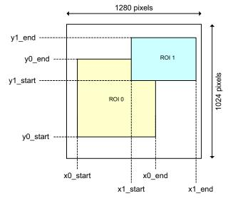
Figure 22. Overlapping Multiple Window Configuration
