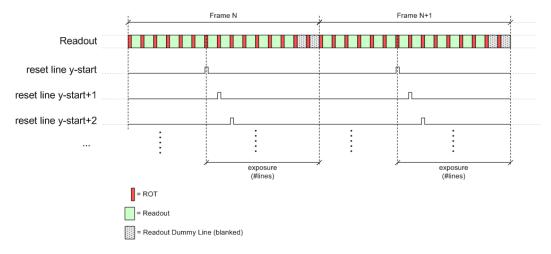
Figure 20. Integration Control in Rolling Shutter Mode
