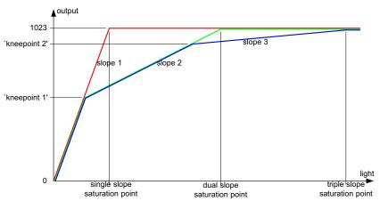
Figure 25. Multiple Slope Operation
