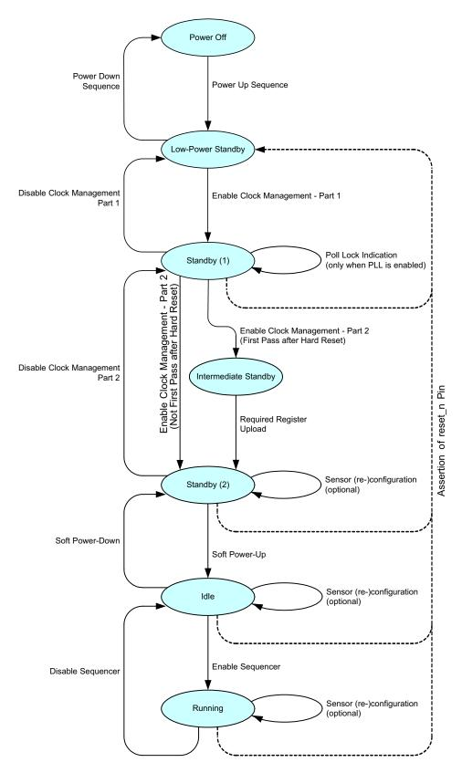
Figure 11. Sensor Operation Flowchart
