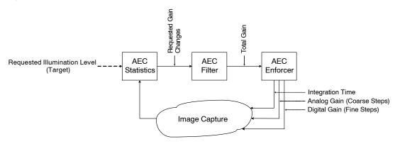
Figure 28. Automatic Exposure Control Loop
