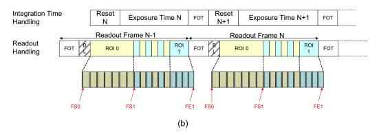
Figure 29. V1-SN/SE: Frame Sync Codes
