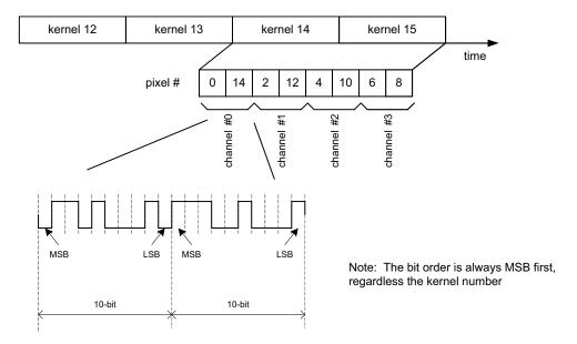
Figure 35. V1-SN/SE: Data Output Order in Subsampling Mode on a Monochrome Sensor
