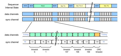
Figure 30. V1-SN/SE: Time Line for Black Line Readout
