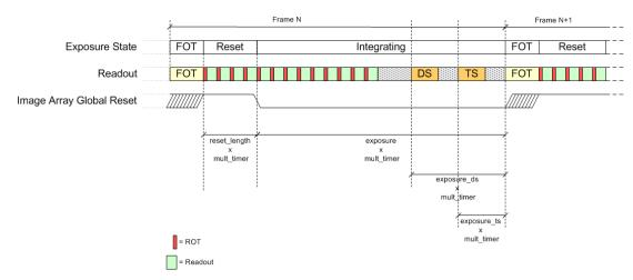
Figure 26. Multiple Slope Operation in Master Mode for fr mode = '0' (Pipelined)
