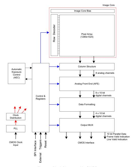
Figure 5. Block Diagram - V2-SN/SE
