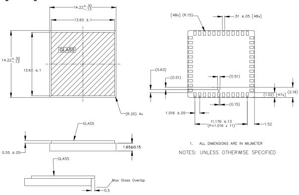
Figure 42. Package Drawing for the 48-pin LCC Package
