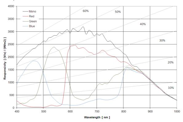
Figure 3. Spectral Response Curve for Mono and Color
