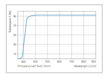
Figure 44. Transmission Characteristics of the Glass Lid
