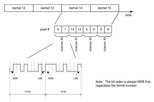
Figure 36. V1-SN/SE: Data Output Order in Subsampling Mode on a Color Sensor
