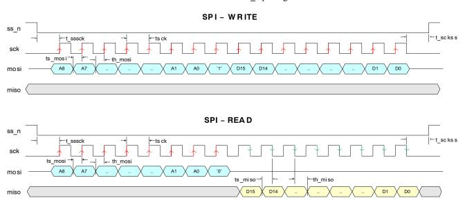
Figure 16. SPI Read and Write Timing Diagram
