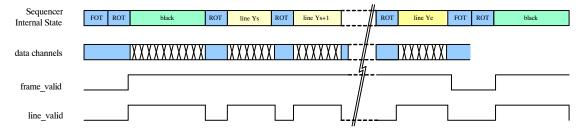
Figure 37. V2-SN/SE: Frame Timing Indication
