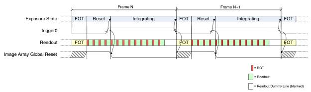
Figure 19. Exposure Time Control in Global-Slave Mode
