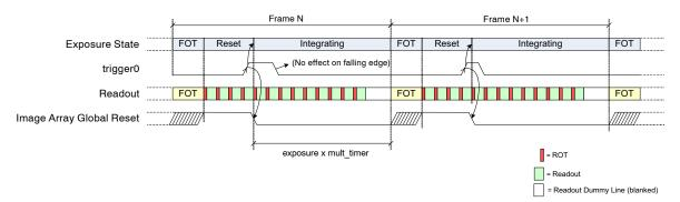
Figure 18. Exposure Time Control in Triggered Shutter Mode (Master)
