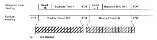
Figure 7. Integration and Readout for Pipelined Shutter
