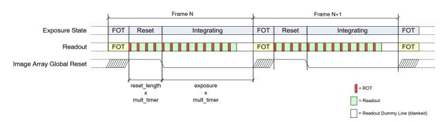
Figure 17. Integration Control for (Pipelined) Global Shutter Mode (Master)
