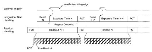
Figure 9. Triggered Shutter Operated in Master Mode
