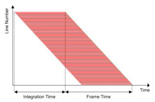
Figure 10. Rolling Shutter Operation
