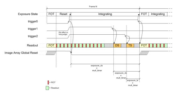
Figure 27. Multiple Slope Operation in Slave Mode
